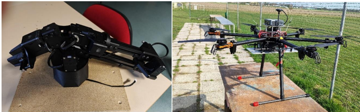
Figure 8: (left) Manipulator used for the UAM (WidowX 250 Mobile arm), (right) Custom UAV platform that will mount the manipulator (Tarot T960 frame).
