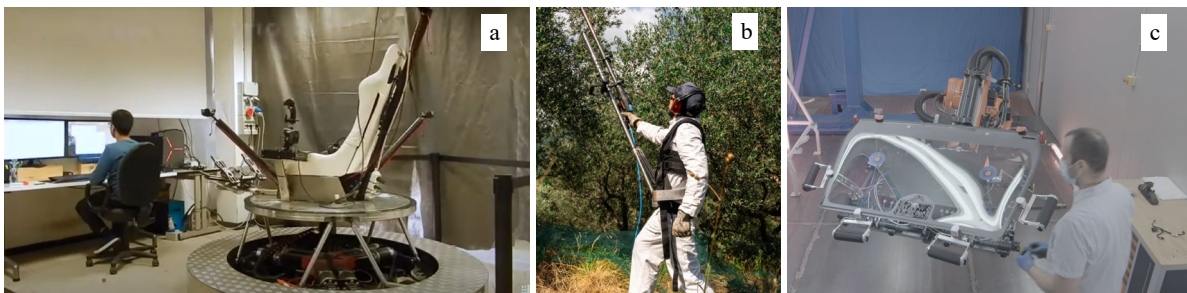
Figure 7: PMAR Lab research prototypes: a parallel robot for motion simulation in VR (a), an exoskeleton for the operation of long tools (b), and a special-purpose end-effector for collaborative assembly of an automotive windshield (c).
